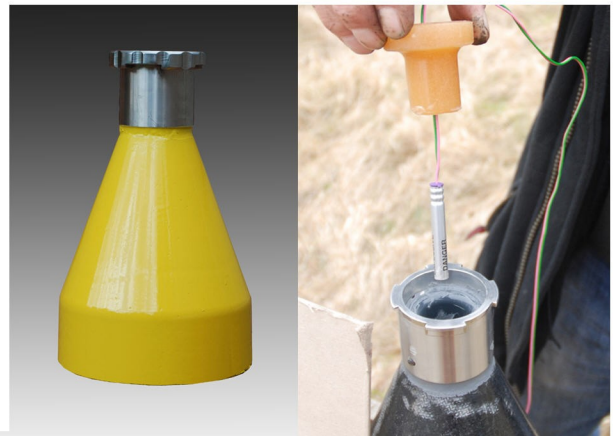
Det Cone - The detonator is placed into the lined chamber and sealed with the rubber moulding before locking in place with the quick action steel cap
