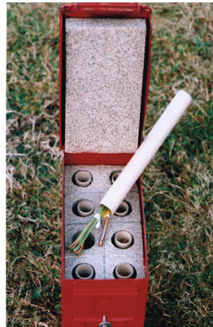
Detsafe 8L, typical electric detonator and fuel fire test used as part of UN certification process
