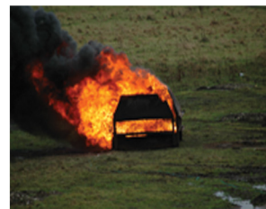
Detsafe 8M, typical electric detonator and fuel fire test used as part of UN certification process
