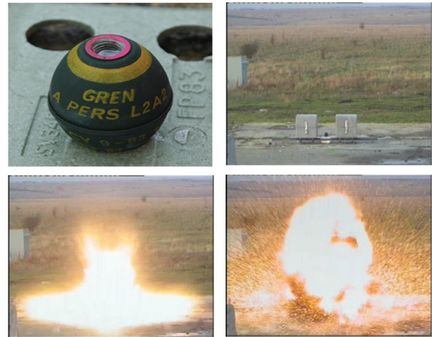
Blast Testing Fuelsafe Units with L2A2 Hand Grenade
