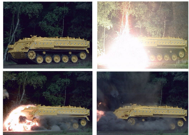
Blast testing of a vehicle protection package to AEP55 Vol 2
