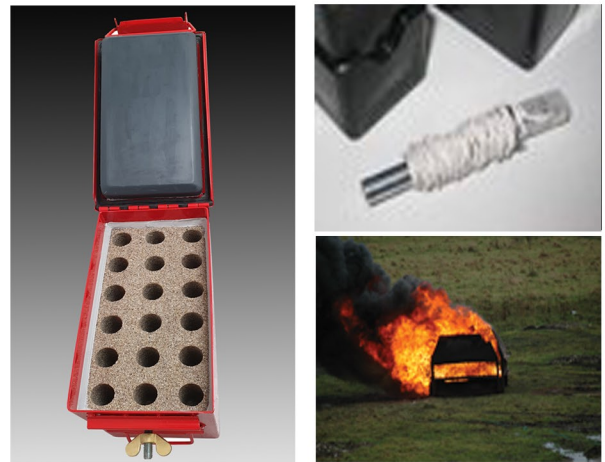
Detsafe 18M, typical electric detonator and fuel fire test used as part of UN certification process.
